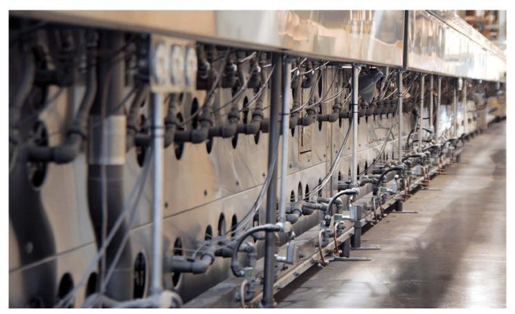
drastically reduce the chance of product and productivity losses due to fires. By far, DGF fires tend to occur in the drying zones toward the end of the oven, where the chance of nearly finished products falling off the belt and collecting near an exposed burner flame is far higher than in the front. The absence of exposed flames in the convection zones helps reduce the risk of fires and makes it easier for operators to keep the product in specification between start-up and shutdown.
