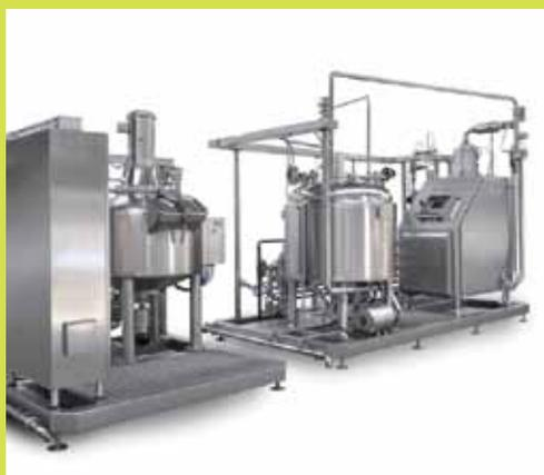
▲ Continuous mixing/aeration systems feature several different pieces of equipment including slurry premixers, buffering tanks and aeration mixers. Pumps are used to transfer the batter to the various pieces of equipment and eventually to a hopper/depositor.
