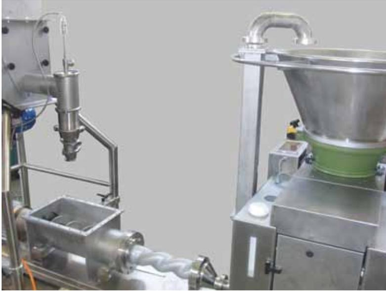
◀ With this continuous mixer, the water jet nozzle on the left hydrates flour, and the dough is developed in the mixing tube, then transferred into the hopper.
