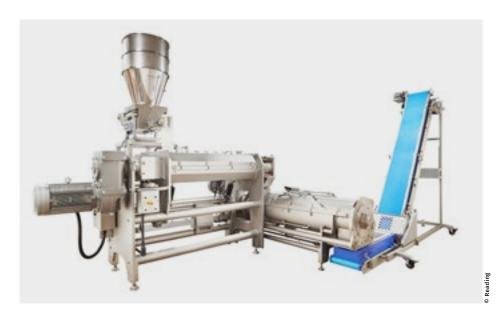
The "high development mixer" is a further development of Reading's mixer family originally developed for snack, cracker and biscuit/cookie lines. The mixer operates in two stages. Two shafts in the first stage blend the raw
