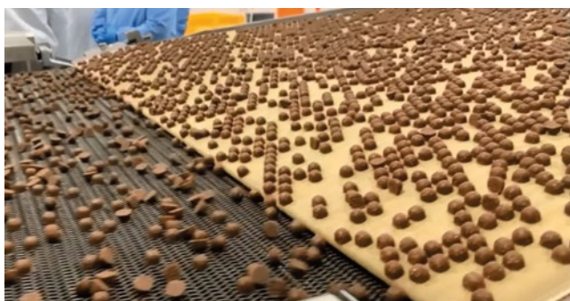
Figure 4: Baked kibble entering the oven in one layer to ensure efficient baking.
