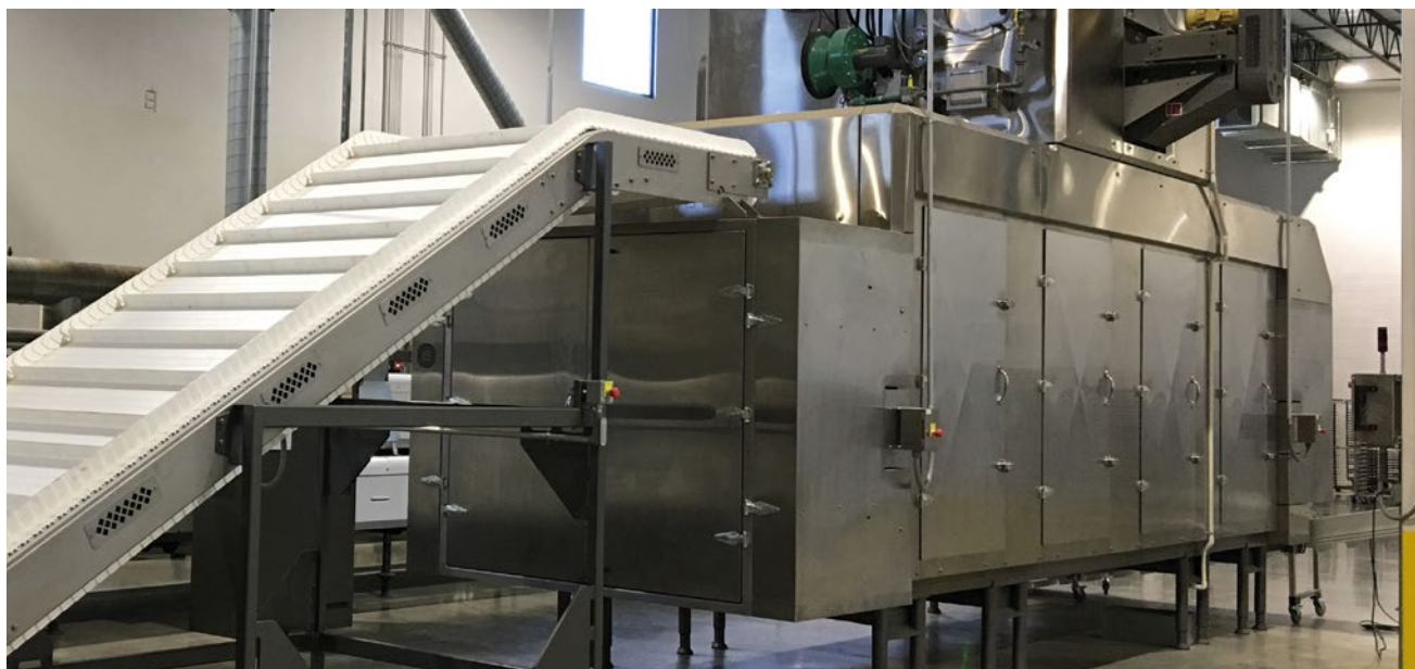
Figure 5: Multi-Pass Dryer for slower drying to gently reduce residual moisture.
